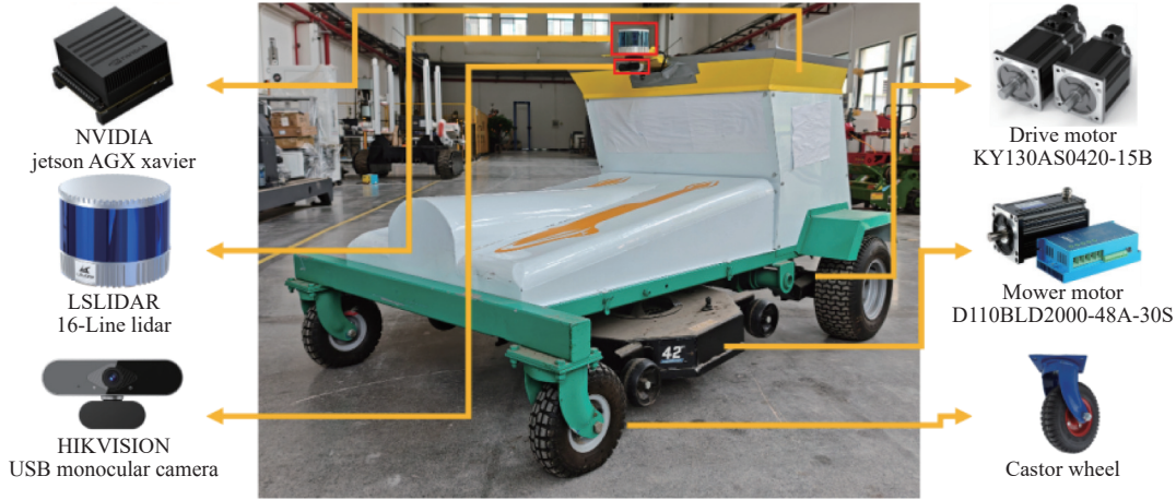
Figure 1 The hardware architecture of an autonomous field mower
