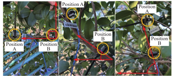
Figure 26 Arrangement positions of acceleration sensors
