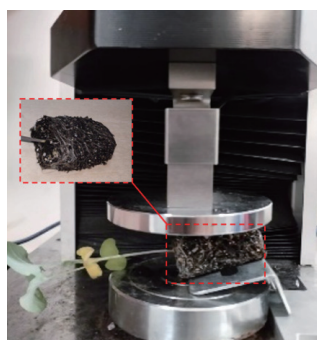
a. Compression test of the root-substrate composite
