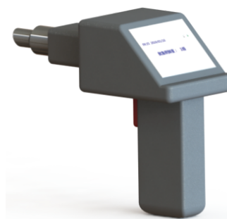
Figure 2 Three-dimensional (3D) structural design rendering of the handheld Vis-NIR spectroscopic detection device
