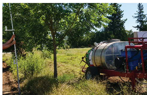
Figure 4 Air velocity measurement positions using cup anemometers at the outer canopy surface during field experiments
