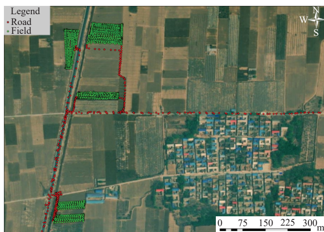
Figure 2 An example of the field-road trajectory segmentation
