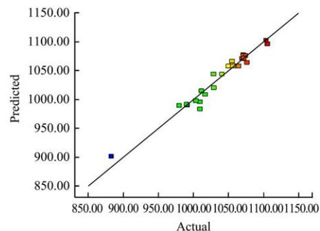
Figure 2c Predicted vs. experimental values of pellet density ( $\text{kg m}^{-3}$ )
