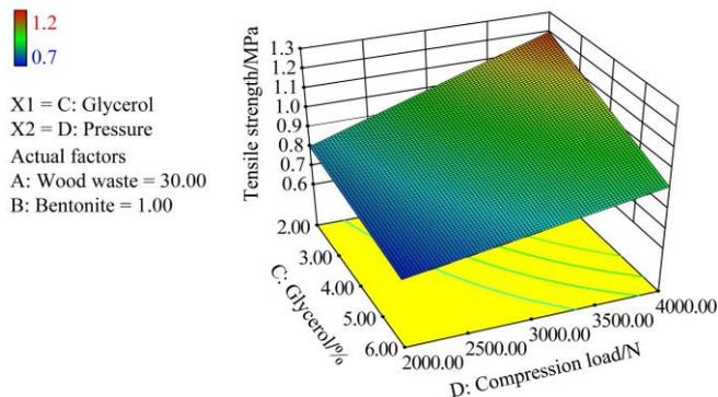
Figure 4 Three-dimensional plot of response surface of pellet tensile strength as function of change in the addition of crude glycerol and compression load (wood residue added at 30% and bentonite added at 1%)
