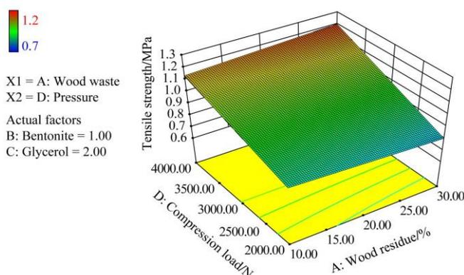
Figure 6 Three-dimensional plot of response surface of pellet tensile strength as function of change in the addition of wood residue and compression load (bentonite added at 1% and crude glycerol added at 2%)
