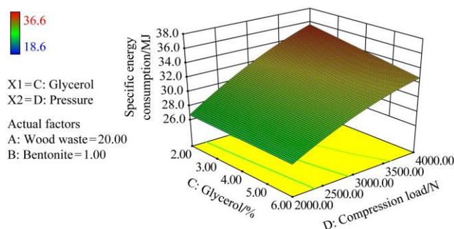
Figure 8 Three-dimensional plot of response surface of specific energy consumption as function of change in the addition of crude glycerol and compression load (bentonite added at 1% and wood residue added at 20%)
