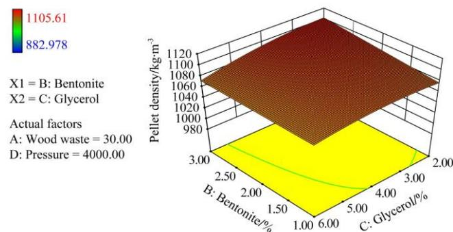
Figure 9 Three-dimensional plot of response surface of pellet density as function of change in the addition of crude glycerol bentonite (wood residue added at 30% and compression load at 4 000 N)
