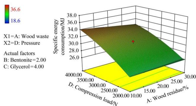
Figure 7 Three-dimensional plot of response surface of specific energy consumption as function of change in the addition of wood residue and compression load (bentonite added at 2% and crude glycerol added at 4%)
