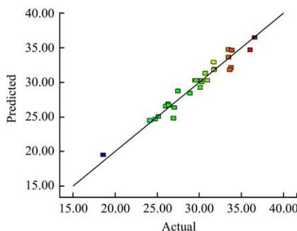
Figure 2b Predicted vs. experimental values of specific energy consumption ( $\text{MJ t}^{-1}$ ) during pelleting
