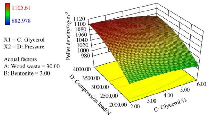
Figure 10 Three-dimensional plot of response surface of pellet density as function of change in the addition of crude glycerol and compression load (bentonite added at 3% and wood residue added at 30%)
