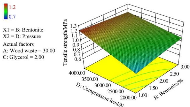
Figure 5 Three-dimensional plot of response surface of pellet tensile strength as function of change in the addition of bentonite and compression load (wood residue added at 30% and crude glycerol added at 2%)
