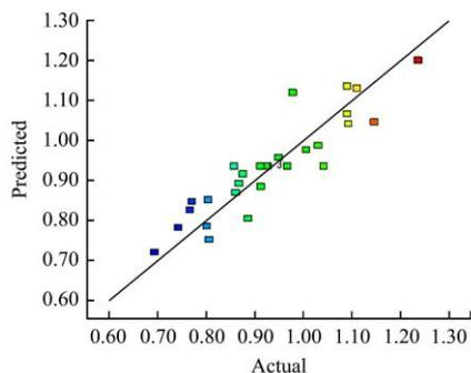
Figure 2a Predicted vs. experimental values of pellet tensile strength (MPa)
