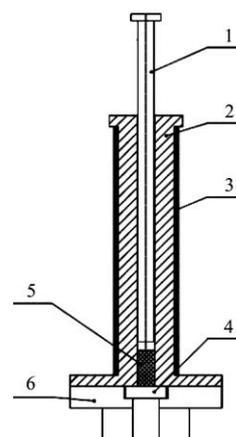
1. Plunger 2. Cylindrical die 3. Heating element 4. Base plate
