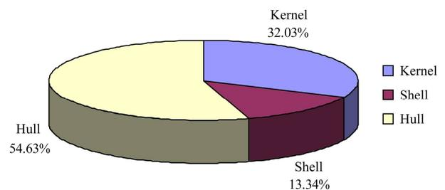
Figure 6 Mass proportions of hull, shell and kernel in an almond
