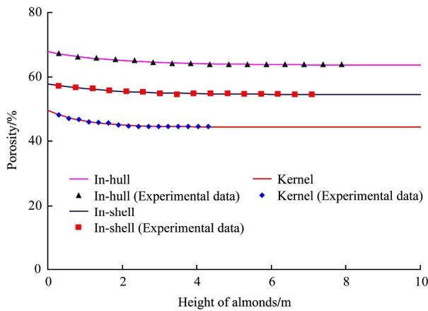
Figure 8 Experimental and modeled results of porosities for different heights of almonds
