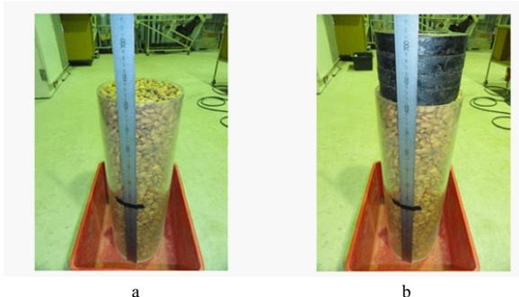
Fig.5 Measuring bulk density with different stockpiling height
