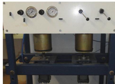
Figure 3 Air-comparison pycnometer
