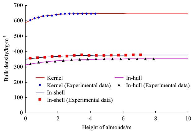
Figure 7 Experimental and modeled results of bulk densities for different heights of almonds
