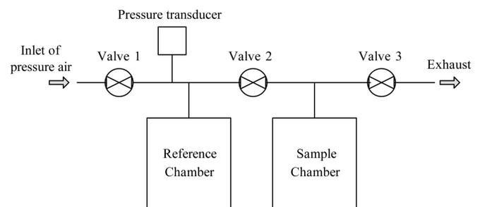
Figure 4 Schematic diagram of an air-comparison pycnometer
