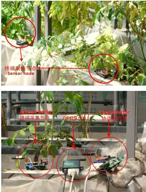
Figure 5 Deployment environment and equipment in experiment
