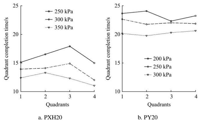
Figure 4 Quadrants completion time through the four quadrants of rotation at varying operating pressures with nozzle size (8 mm)
