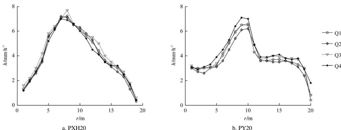
Figure 6 Average water application patterns in the quadrants for the PXH20 and PY20 sprinklers with nozzle size of 8 mm at 300 kPa
