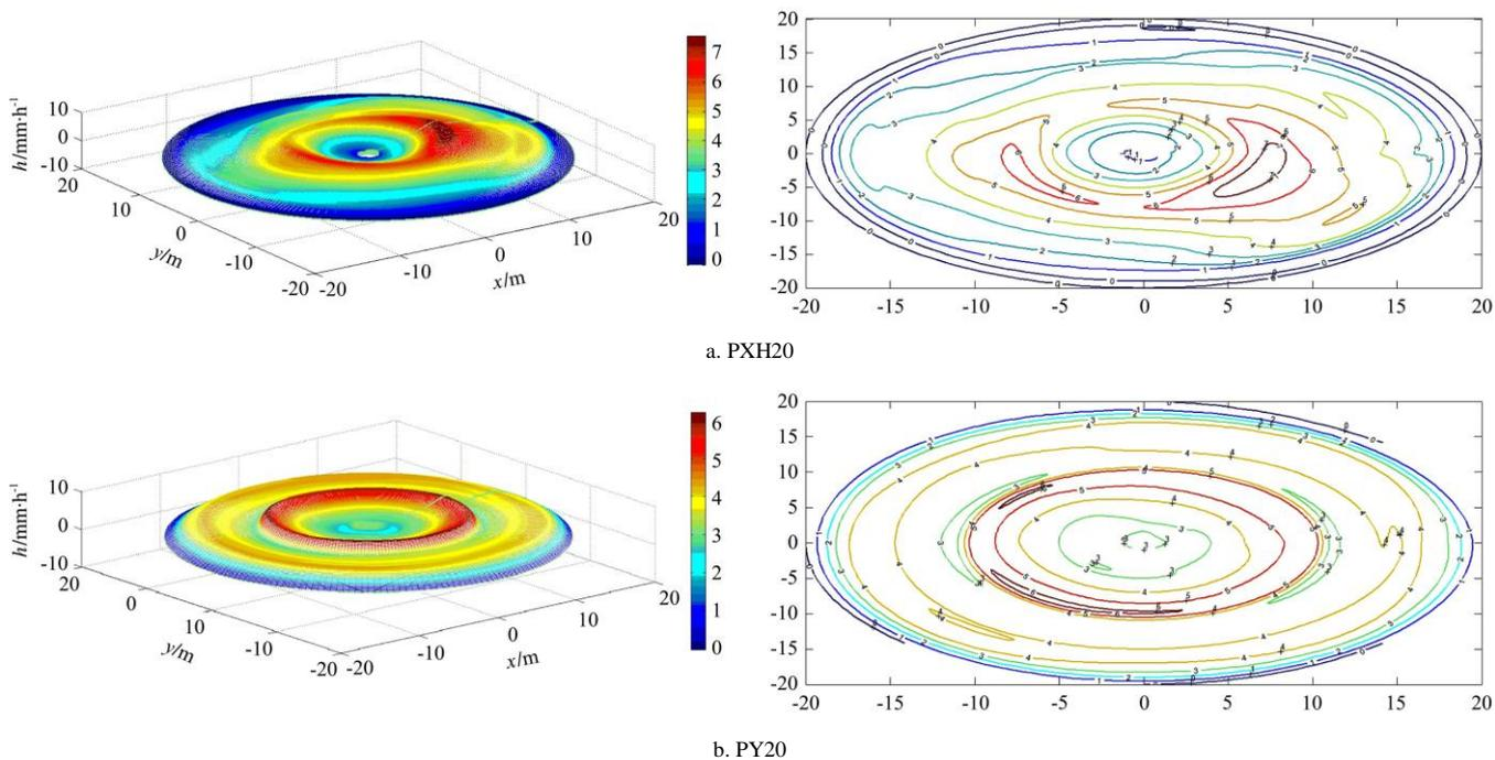
Figure 7 Sample water application pattern for the PXH20 and PY20 sprinklers with nozzle size of 8 mm at 300 kPa. The color bars indicate the water application rate
