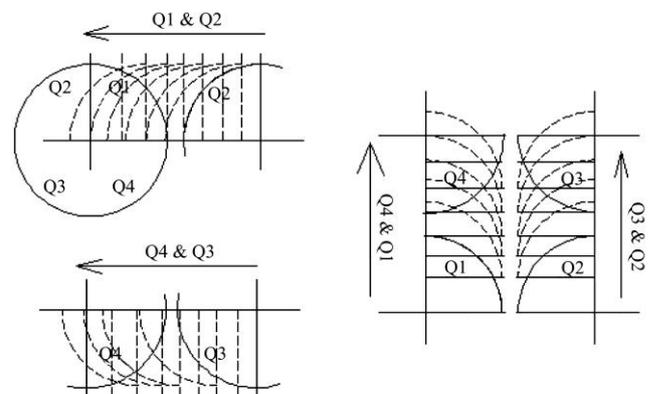
Figure 3 Schematic view of overlap of quadrants for a complete single sprinkler coverage area
