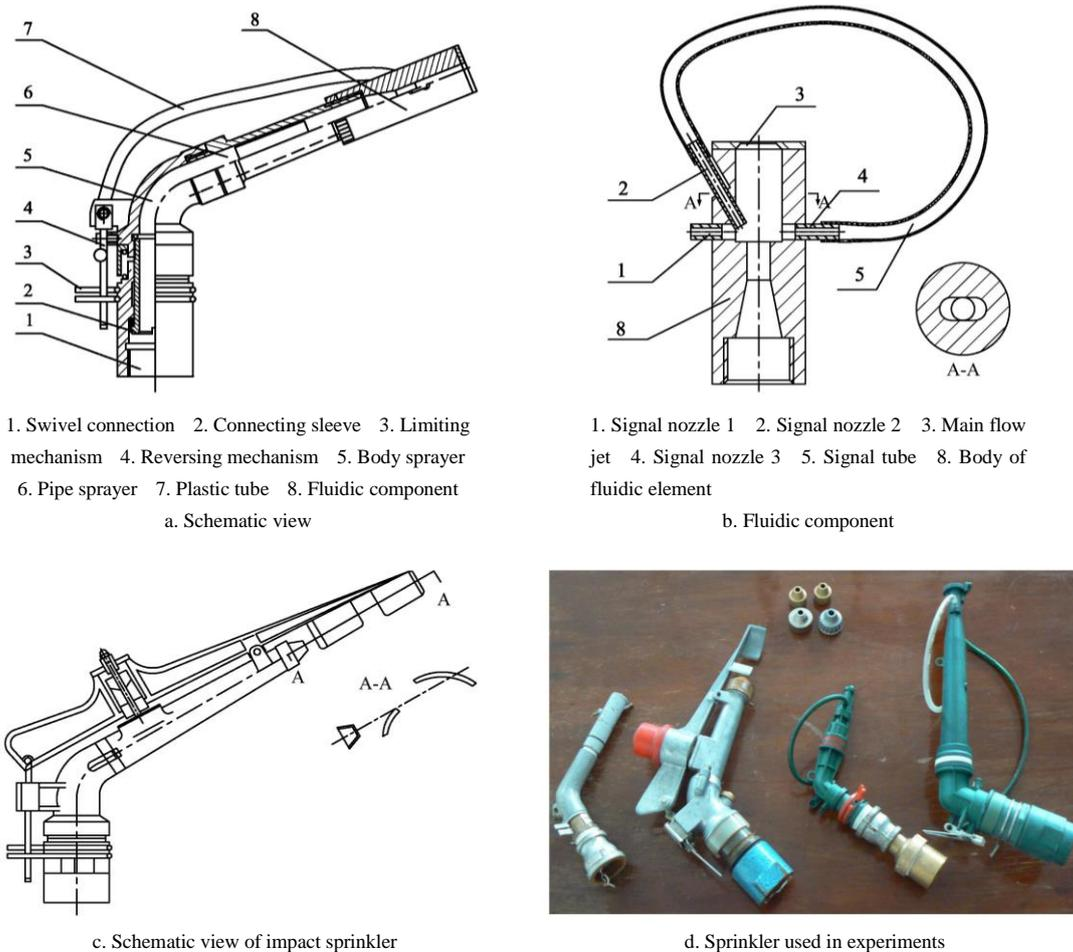
Figure 1 Schematic and pictorial views of fluidic and impact sprinklers used in the experiment
