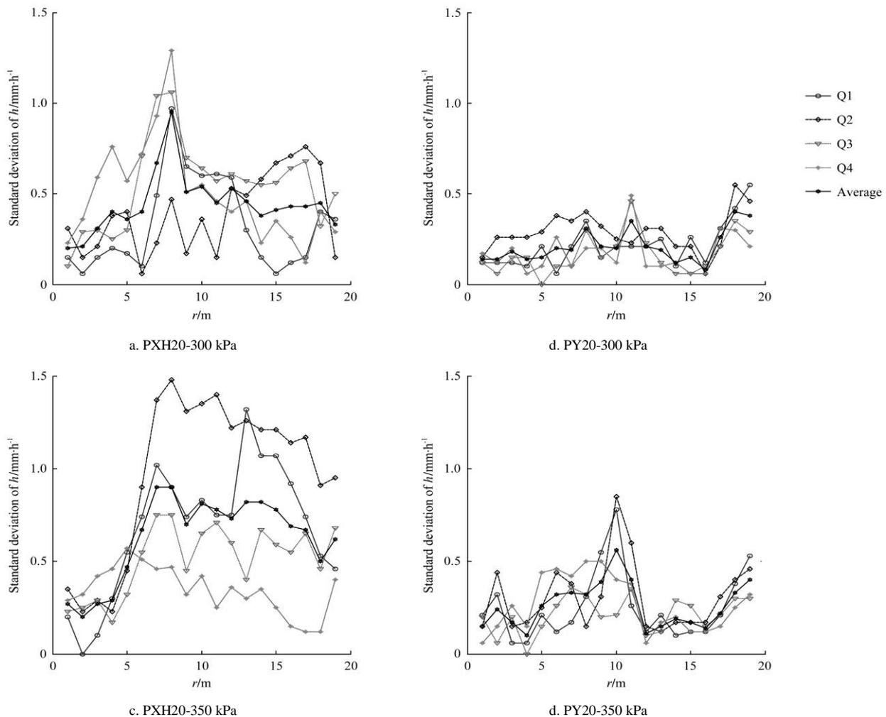
Figure 8 Standard deviation of water application rate against distance from sprinkler within quadrants
