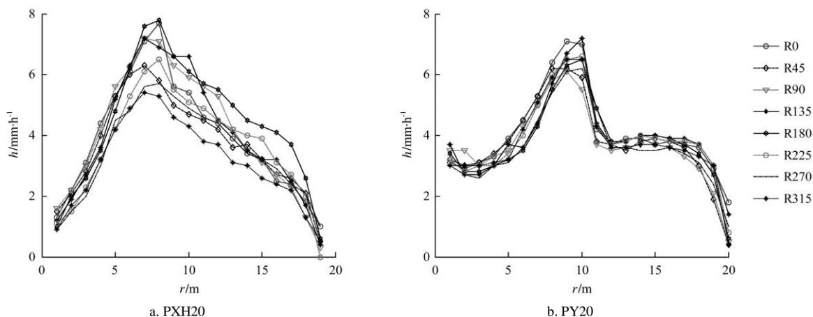
Figure 5 Radial leg data along eight radial lines for the PXH20 and PY20 sprinklers with nozzle size of 8 mm at 300 kPa
