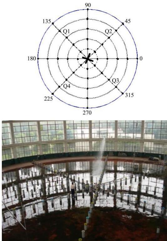
Figure 2 Schematic and pictorial views of layout of cans around sprinkler in the indoor laboratory
