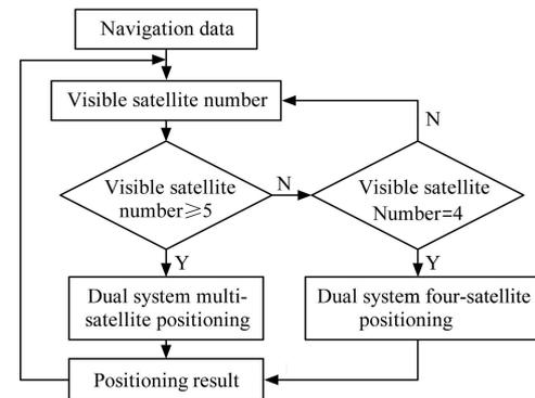
Figure 1 Structure diagram of BDS/GPS Integrated Positioning
