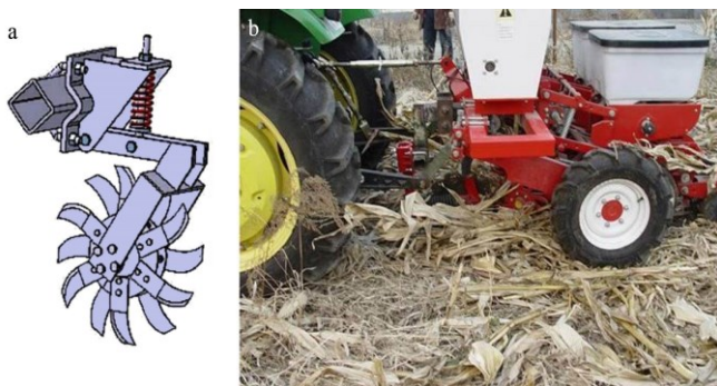
Figure 9 (a) Schematic diagram of sliding-knife notched disc opener [62] and (b) Passing through straw mulching area
