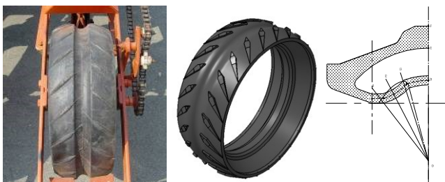
Figure 6 Press wheel and sketch of the cavity's section [60]
