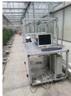
Figure 10 The developed measurement platform
