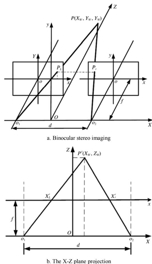
Figure 1 Schematic diagram of a stereo vision system
