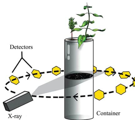
Figure 1 Illustration of the principle of CT in imaging slices of plant soil<sup>[43]</sup>
