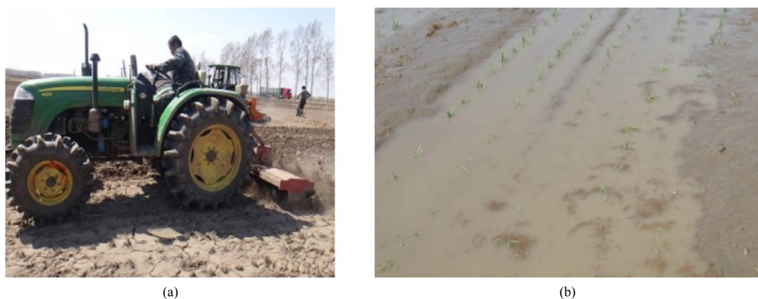
Figure 3 (a) Photograph of locally available rotavator for full tillage dry land preparation. (b) Young plants transplanted by conventional mechanization systems in treatment T2
