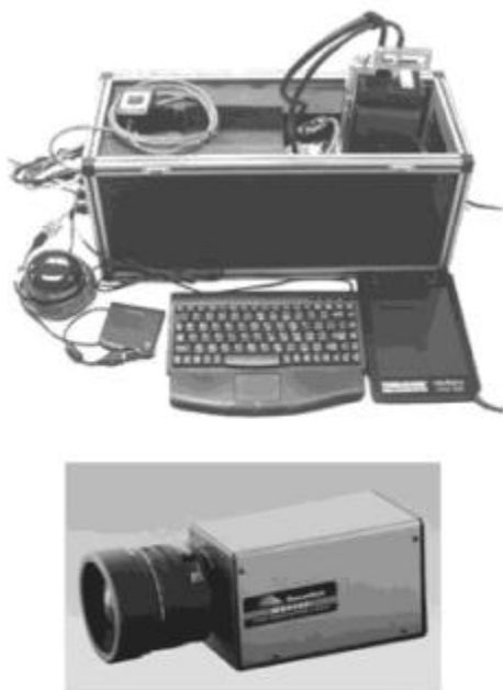
Figure 2 TerraHawk aerial imaging system and MS4100 multispectral camera
