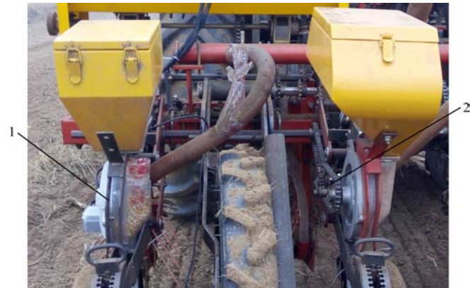
1. Mechatronic driving system 2. Ground wheel and chain-sprockets driving system
