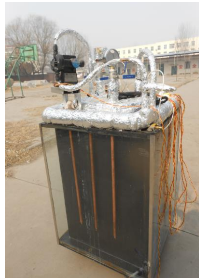
Figure 6 Diagram of the new biogas fermentation system by solar heat pipe heating
