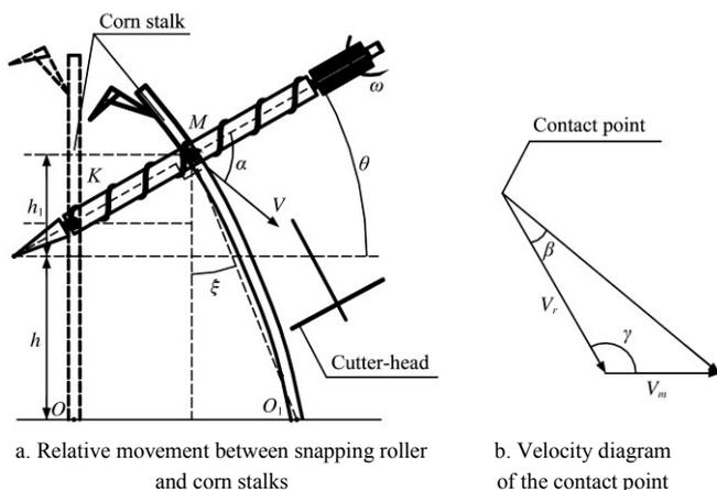
Figure 2 Sketch map of effect between corn stalks and the snapping roller
