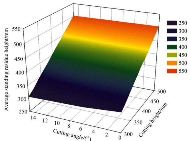
Figure 7 Relationship among average SRH, cutting height and cutting angle
