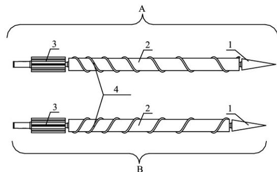
A. Outer snapping roller B. Inner snapping roller 1. Tapering portion
