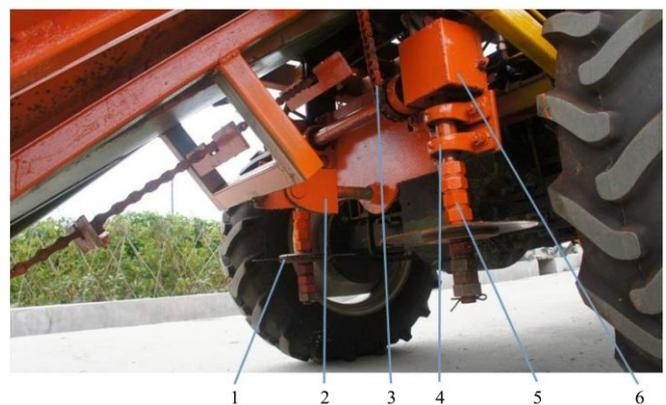
1. Cutter-head 2. Adjust mechanism of cutting angle 3. Driving chain
