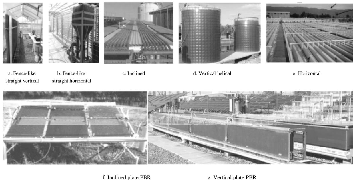
Figure 2 Different designs of tubular and plate PBRs (a and b: courtesy of L. Thomsen, Jacobs University, Germany; c, d, e: courtesy of M. R. Tredici<sup>[26]</sup>, University of Florence, Italy; f: courtesy of A. Richmond<sup>[38]</sup>, BenGurion University, Israel; g: courtesy of Q. Hu and M. Sommerfeld<sup>[7]</sup>, Arizona State University)
