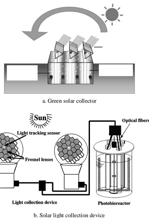
Figure 4 Different solar collectors (a: courtesy of Zijffers et al.; b: courtesy of Ogbonna et al.<sup>[53]</sup>)
