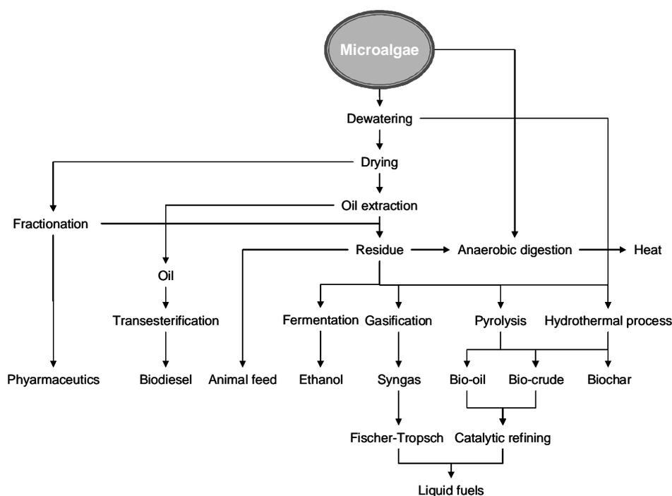
Figure 7 An integrated biorefining scheme for algal biomass utilization
