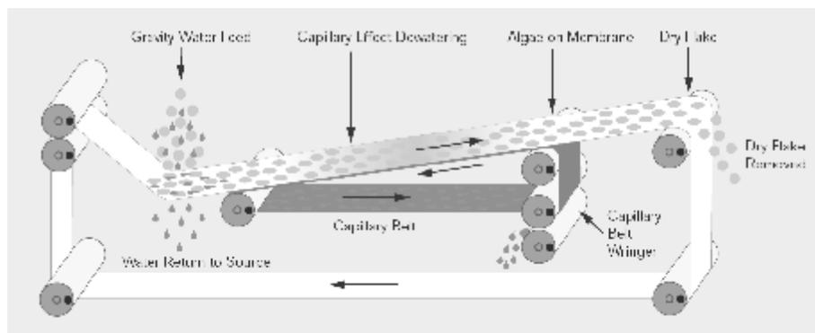
Figure 5 AlgaeVenture harvest, dewatering, and drying system
