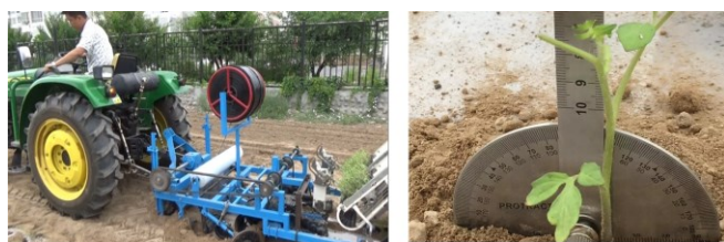
a. Field test of the seedling transplanter b. Test of seedling perpendicularity
