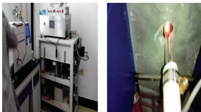
Figure 14 Hydrogen came into being when the inside pressure was over 0.7 atm.
