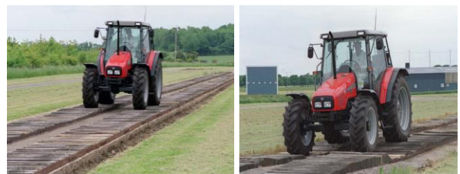
Figure 1 ISO100-m smooth track (left) and ISO35-m rough track
