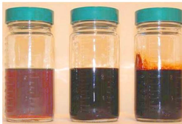
Figure 3 Picture of light oil, heavy oil and bio-oil from left to right
