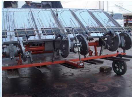
The first wide-narrow-row riding-type rice transplanter was developed successfully in May, 2010, with the photos of tests in the field.
