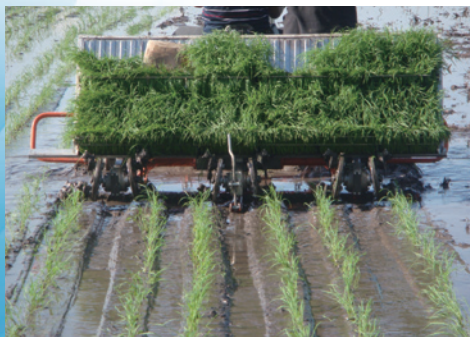
The first wide-narrow-row riding-type rice transplanter was developed successfully in May, 2010, with the photos of tests in the field.
