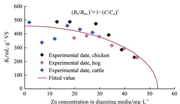
Figure 4  $B_0$  as function of Zn concentration
