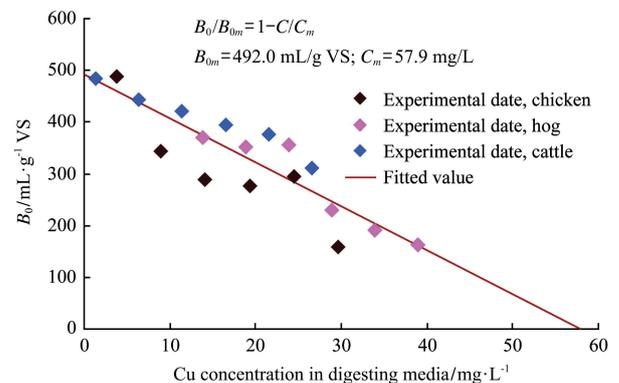
Figure 3  $B_0$  as function of Cu concentration
