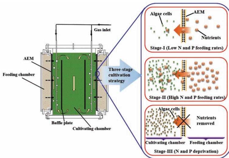
Figure 1 Schematic of anion exchange membrane photobioreactor and the process of three-stage cultivation strategy<sup>[16]</sup>
