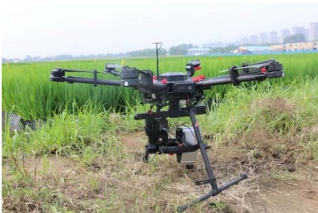
Figure 2 UAV-M600 and Gaiasky-mini hyperspectral imaging camera
