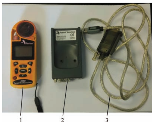
1. Host of Kestrel 4500 2. Data reading terminal-Kestrel Interface 3. Data cable Figure 4 Anemometer and related components
