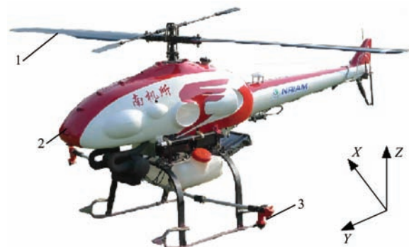
1. Rotor 2. Fuselage 3. Centrifugal atomization nozzles Figure 1 Unmanned agricultural helicopter, N-3
