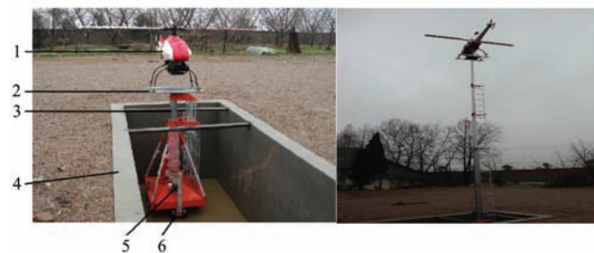
1. UAH 2. Work platform 3. Hydraulic telescopic column 4. Cement geosynclines 5. AC motor 6. Direction traction and handle
