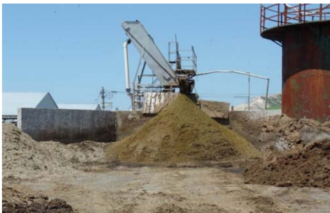
Figure 1 Slurry separation by inclined screen and screw press
