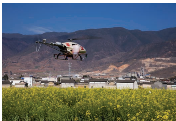
c. 3WQF125-16 UAV spraying on cole by Quanfeng Aviation Plant Protection Technology Co., LTD
