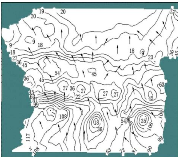
Figure 7 Groundwater flow field and direction in the Manas River irrigation area (Dec 31, 2013)
