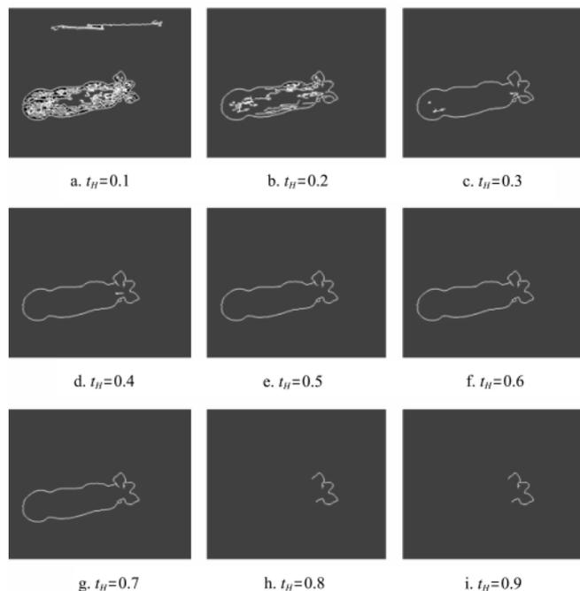
Figure 5 Pig edge images changed with the threshold value  $t_H$
