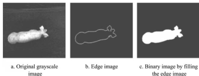
Figure 4 Illustration of pig area extraction based on the edge-detection technique.
