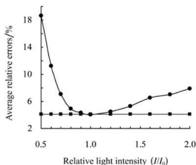
Figure 7 Average relative errors of pig weight estimation vs. simulated relative light intensity of the environment by the conventional method (circle) and the edge detection method (square).
