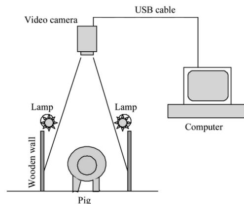
Figure 1 Schematic diagram of the experimental setup used in this study.
