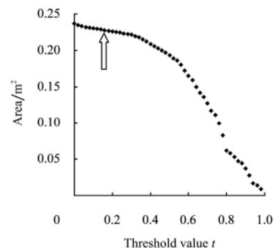
Figure 3 Pig area extracted by converting grayscale image to binary image as a function of the threshold value. The arrow in the figure indicates the corresponding threshold value in the edge detection method
