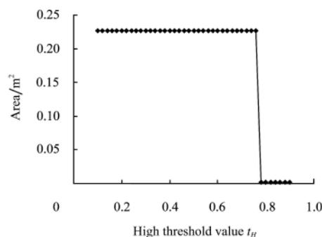
Figure 6 Pig area extracted using Canny edge-detection method as a function of the high threshold value in the edge-detection. The low threshold value  $t_L$  was set to be  $0.4 * t_H$
