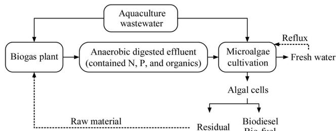
Figure 1 Flow chart of the coupling system that combining microalgae production with effluent treatment
