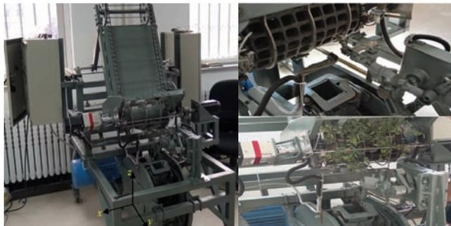
Figure 11 Automatic transplanting test of tomato pot seedlings
