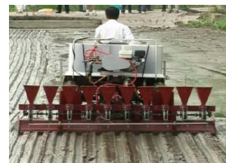
c. PRHDD machine with synchronous spraying
