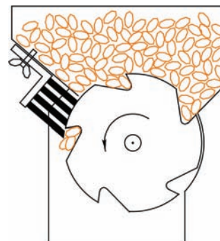
Figure 4 Schematic view of roller-type metering device
