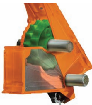
Figure 2 Schematic view of control seed wheels
