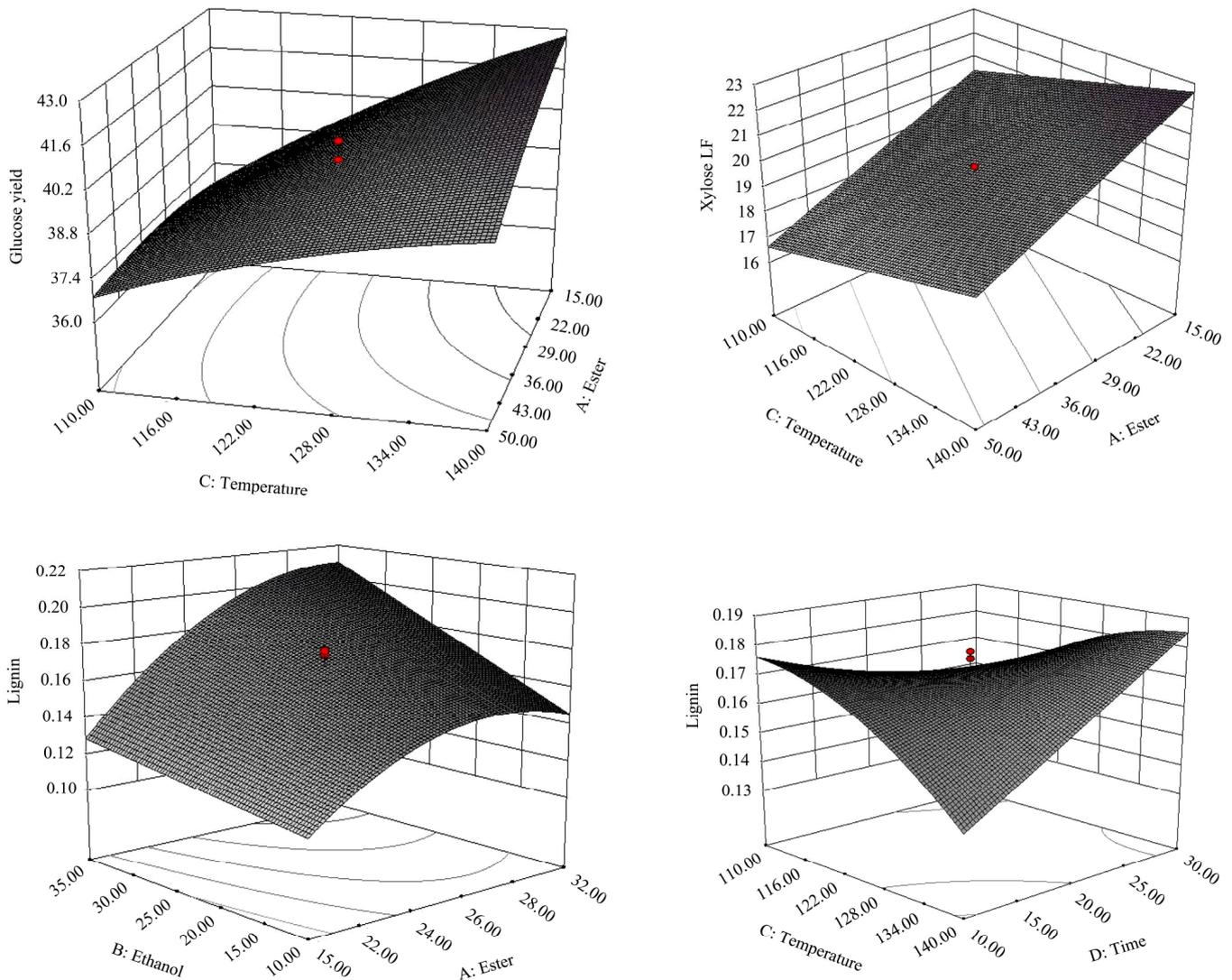
Figure 1 Response surface graphs for glucose yield, xylose recovery and lignin recovery in clean fractionation
