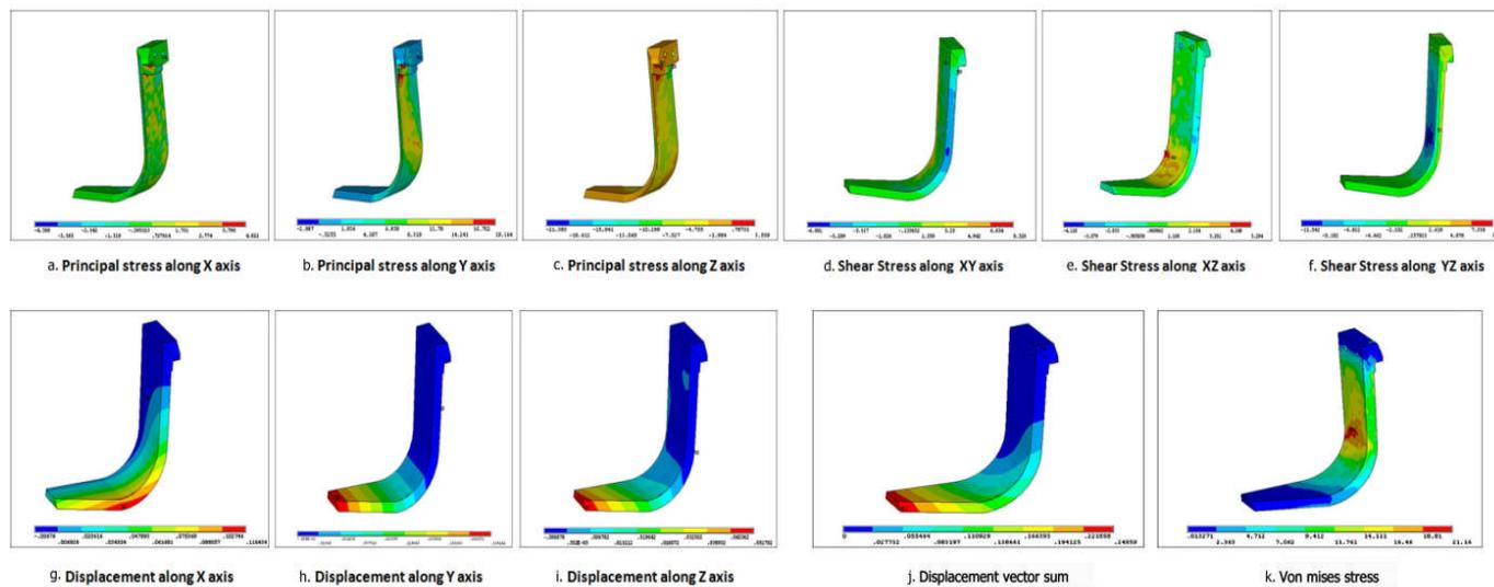
Figure 3 The principal stresses on blade component
