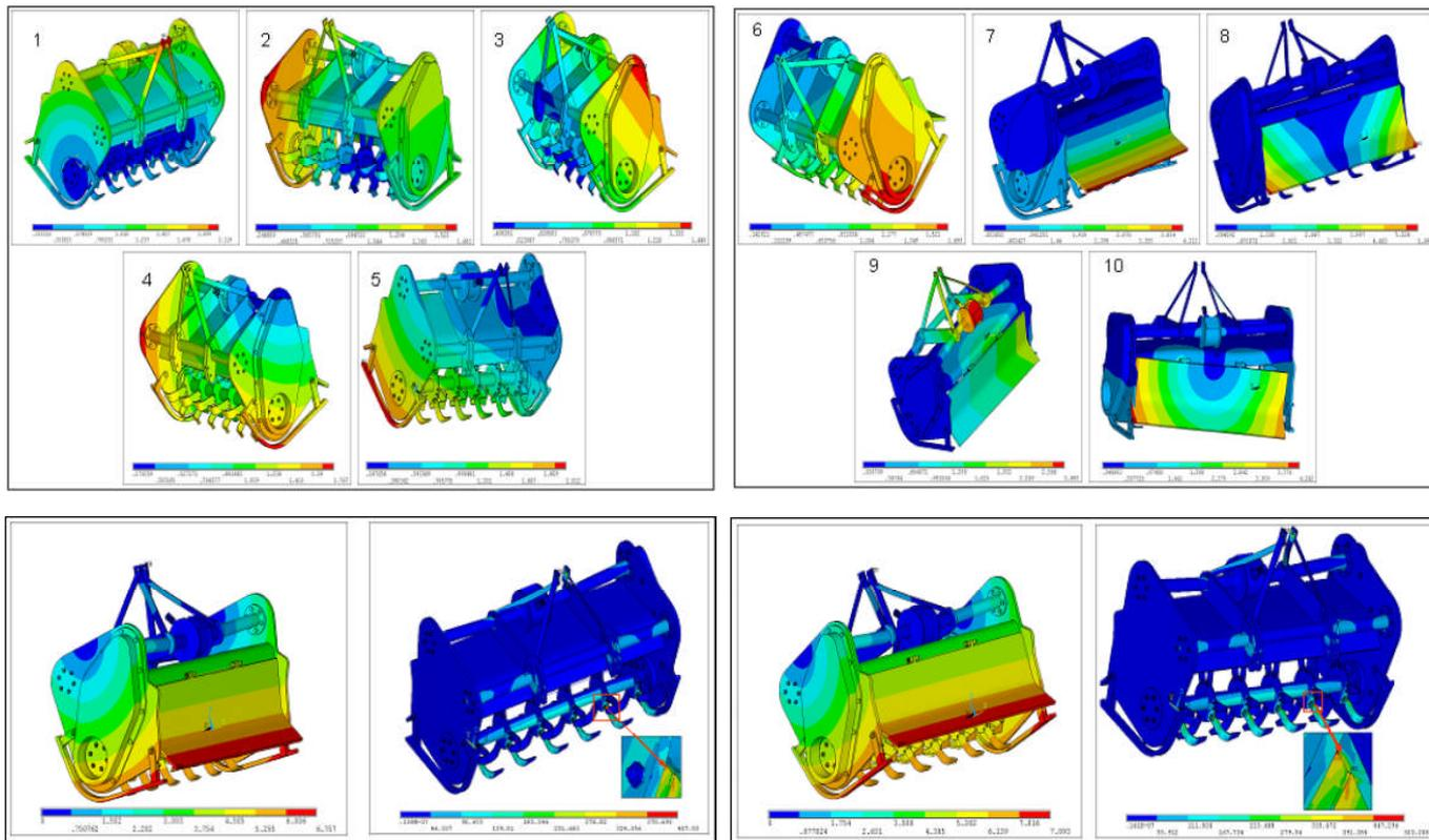
Deformation and stress plot for 35 hp tractor
