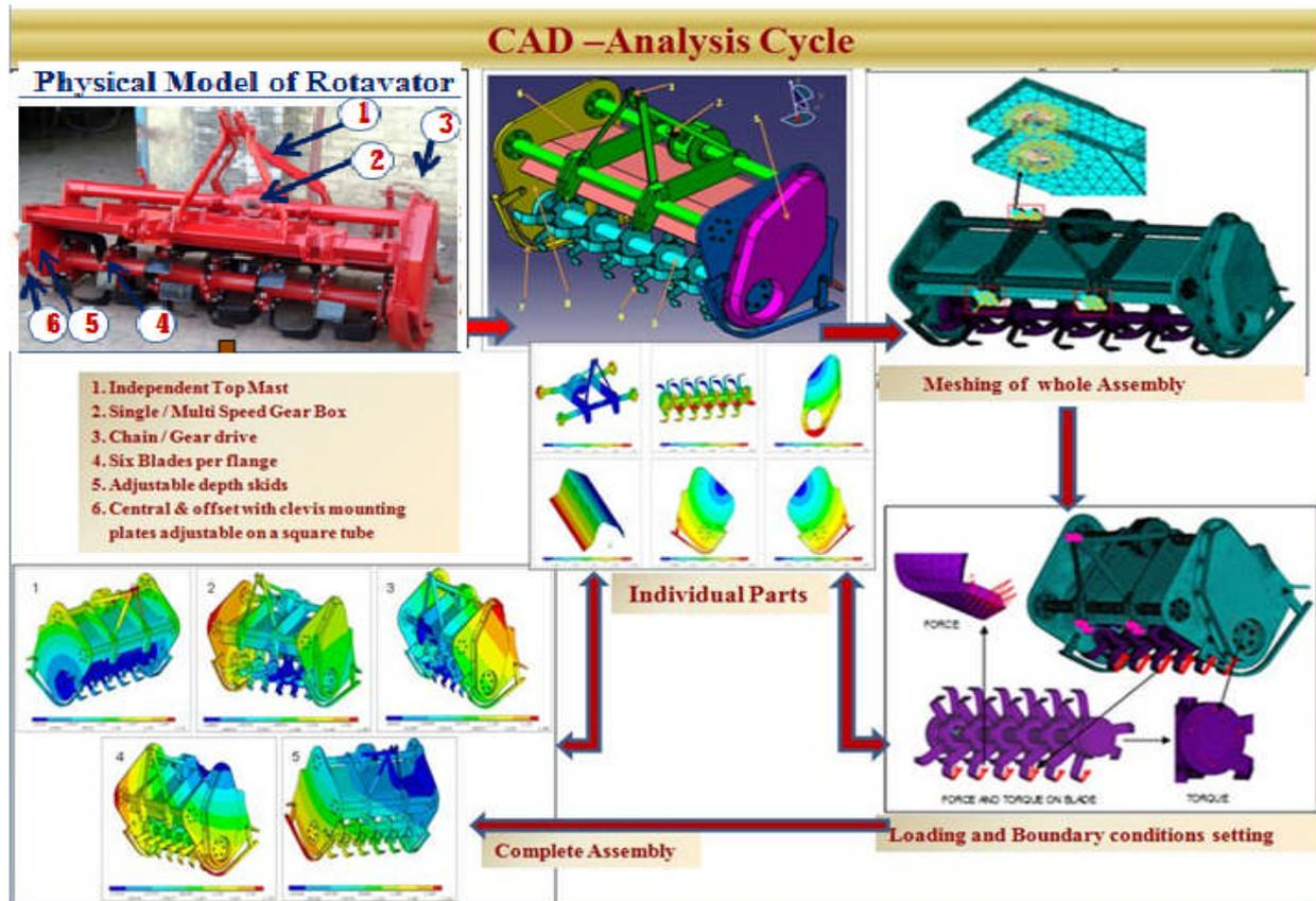
Figure 4 The CAD-analysis cycle
