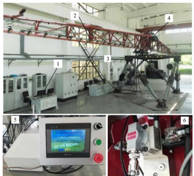
1. Console 2. Proximity sensor 3. Six degrees of freedom motion simulator 4. Spray boom with the pendulum suspension 5. DSP control system and human-computer interface 6. Servo valve
