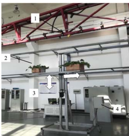
1. Ultrasonic sensor 2. Pot plants 3. Step motor 4. Control cabinet
