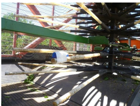
a. Mediolive prototype equipped with nylon rods
