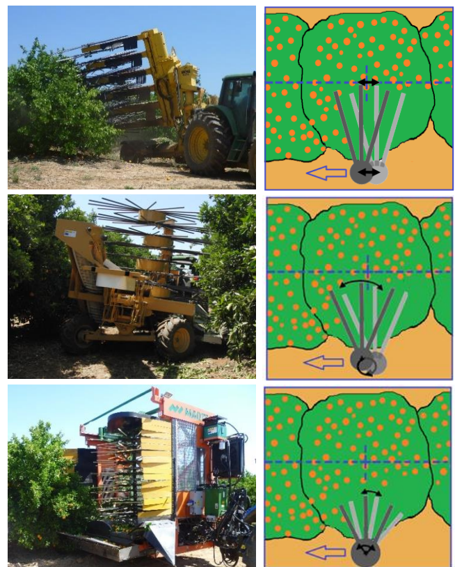
Figure 1 Tractor-drawn citrus harvesters (left) and canopy shaker mechanism descriptions (right) tested for a lateral harvesting of the trees. Oxbo 3210 (top), Samolive (center) and Mediolive (bottom)
