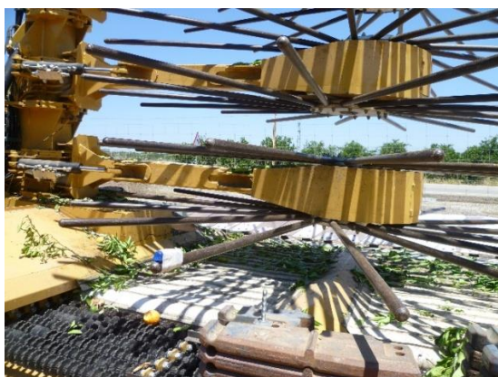
b. Samolive prototype equipped with metal rods
