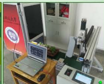
Device for identification and elimination of strong and inferior vegetable potted seedlings
