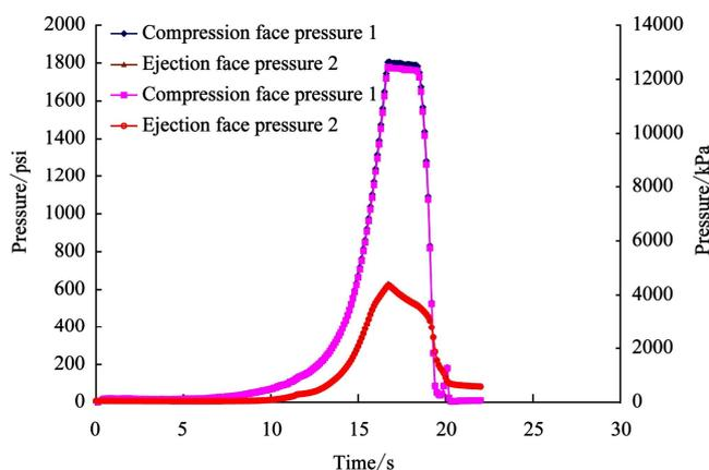
Figure 4 Typical pressure exerted on hay by the main compression and ejection rams over the duration of a test. Pressure 1 was measured by pressure transducer 1 in the compression face; Pressure 2 was measured by pressure transducer 2 in the ejection face
