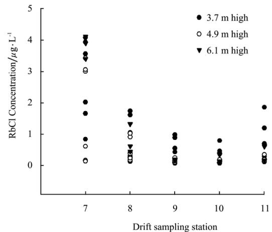
Figure 3 Concentration of RbCl on Mylar as a function of drift sampling station location pooled across all other variables
