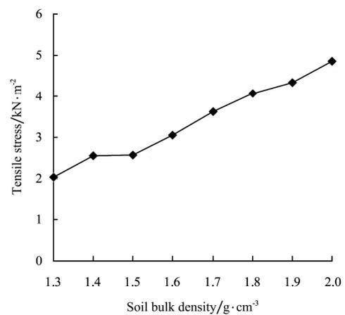
Figure 11 Effect of soil bulk density on tensile stress on hitch bar
