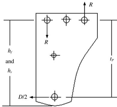
Figure 3 Dimensions and forces on side plates
