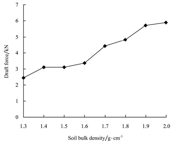
Figure 5 Effect of soil bulk density on draft force
