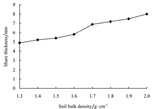
Figure 6 Effect of soil bulk density on share thickness
