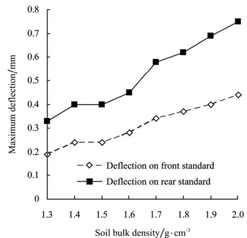
Figure 8 Effect of soil bulk density on maximum deflection on standards
