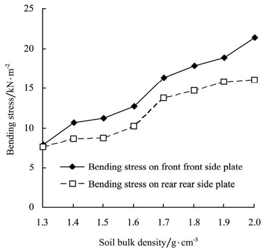
Figure 9 Effect of soil bulk density on bending stress on side plates
