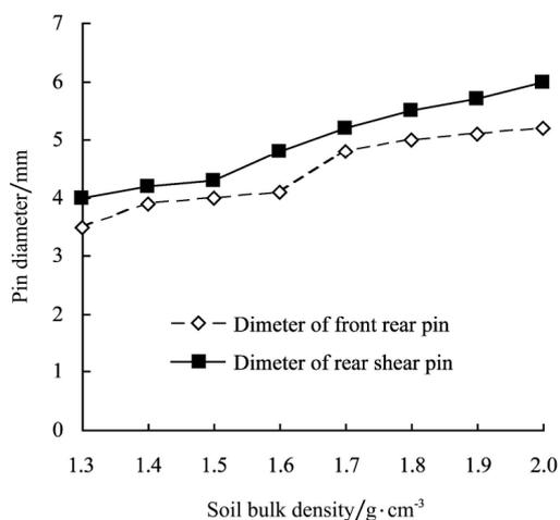
Figure 10 Effect of soil bulk density on diameter of shear pin
