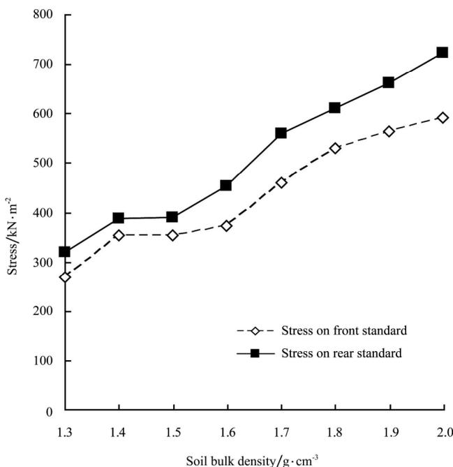
Figure 7 Effect of soil bulk density on stresses on standards
