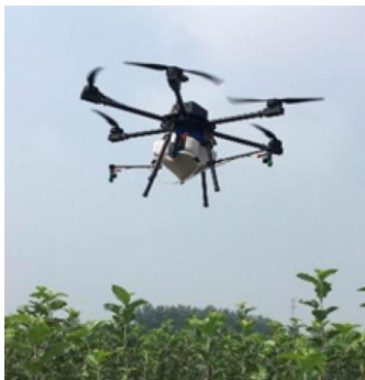
Figure 3 Real-used six-rotor UAV, JF01-10
