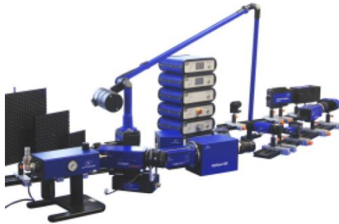
Figure 2 PIV used in the tests
