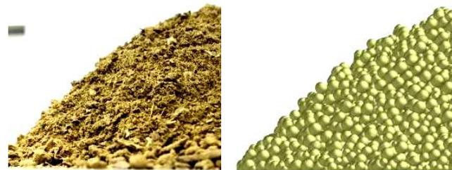
b. Comparison of angle of repose physical test and simulation test of particulate material with water content of (14.2±2.1)%
