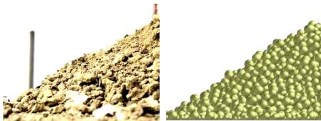
a. Comparison of angle of repose physical test and simulation test of the particulate material with a water content of (6.26±1.5)%
