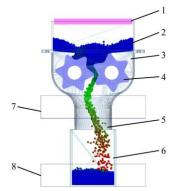
1. Particle factory2. Urea particle3. Fertilizer-board4. The arc gears thatdischarges fertilizer5. The box of fertilizer apparatus6. Particle collector7. Grid bin group (a)8. Grid bin group (b)
