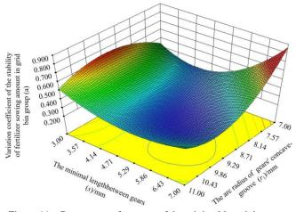
Figure 11 Response surface map of the minimal length between gears (*s*) and the arc radius of gears' concave-groove  $(r_1)$  to variation coefficient
