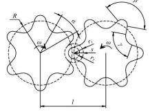
Figure 4 Graphic of design parameters of fertilizer apparatus Among them, the minimal length between gears (*s*) is:
