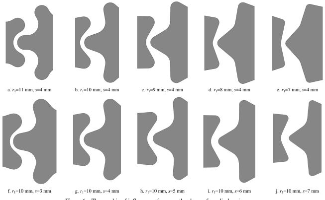
Figure 6 The graphic of influences of  $r_1$ , s on the shape of arc discharging gears
