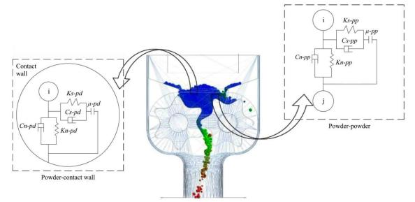
Figure 2 Simplifying treatment of soft-sphere model to contact forces between particles (or particle and wall)
