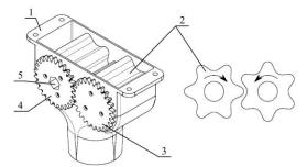
1. Shell 2. Arc discharging gears 3. Driven gear shaft 4. Initiative gear shaft 5. Initiative six-party shaft hole
