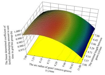
Figure 12 Response surface map of the minimal length between gears (*s*) and the arc radius of gears' concave-groove ( $r_1$ ) to coefficient of determination
