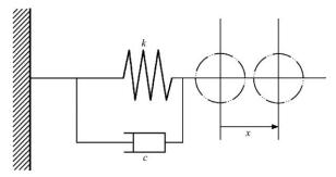
Figure 1 System of spring, damping and oscillator
