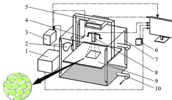
1. Dema frequency converter 2. Fan 3. Omron temperature controller 4. PT100 temperature sensor 5. Electronic balance 6. Single chip microcomputer 7. Infrared heating tube 8. CCD industrial camera and lens 9. Plates 10. Solenoid valve
