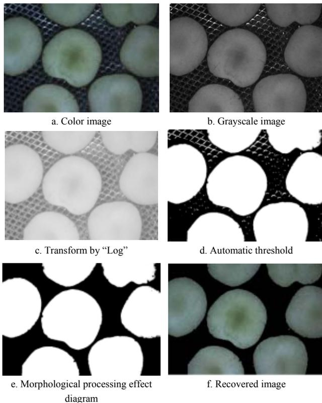
Figure 3 Image processing process of jujube slices in the drying process
