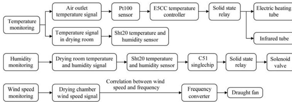
Figure 2 Hardware structure of temperature, relative humidity, and wind speed monitoring
