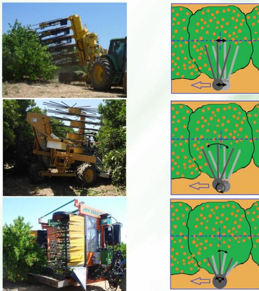
Figure 1 Tractor-drawn citrus harvesters (left) and canopy shaker mechanism descriptions (right) tested for a lateral harvesting of the trees. Oxbo 3210 (top), Samolive (center) and Mediolive (bottom)
