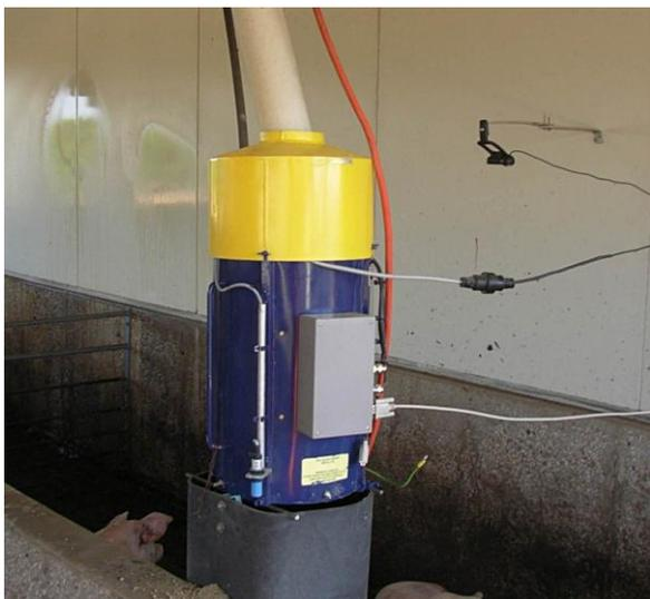
Figure 4 Prototype feed sensor and the camera system undergoing testing at a commercial piggery site<sup>[22]</sup>
